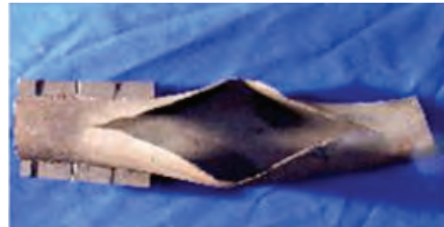
Figure 9.2.11. Boiler tube – failure (rupture)
