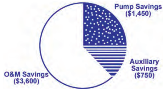
Figure 9.9.6. Pump system energy use and savings.
