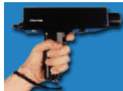
Typical hand-held ultrasonic detector
