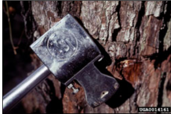
Hypo-Hatchet® showing hole in bit where herbicide is injected. Photo by Gerald J. Lenhard, Bugwood.org.
