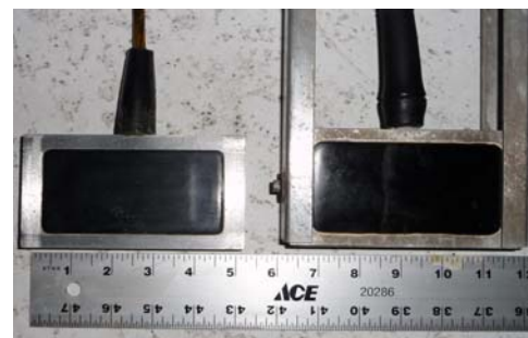
Figure 2. The prototype projectors are ruggedized encased in 5" long x 3" high x 1" thick aluminum blocks. Each projectors consists of 45 ceramic elements that radiate on an axis source level of ~200 dB at both 210 kHz and 225 kHz, producing a narrow directional beam width of about six degrees.
