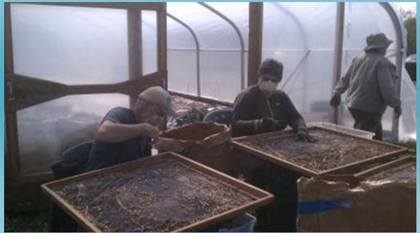
Fig. 16. Hand screening is usually required after using the hammermill.
