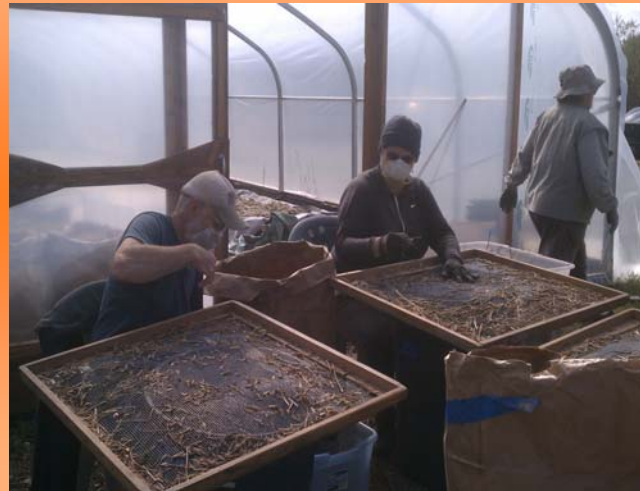
Fig. 22- Hand screening is usually required after using the hammermill
