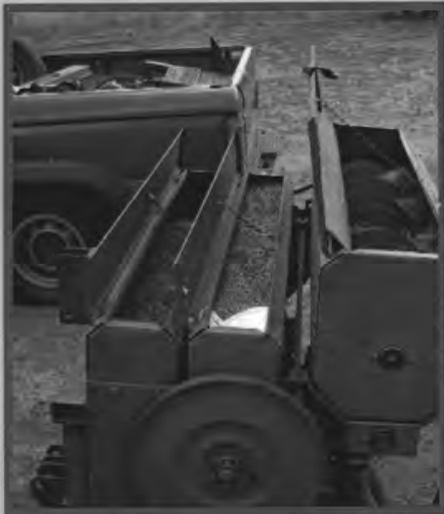
The no-till drill we used had three different bins separating seed by size.
