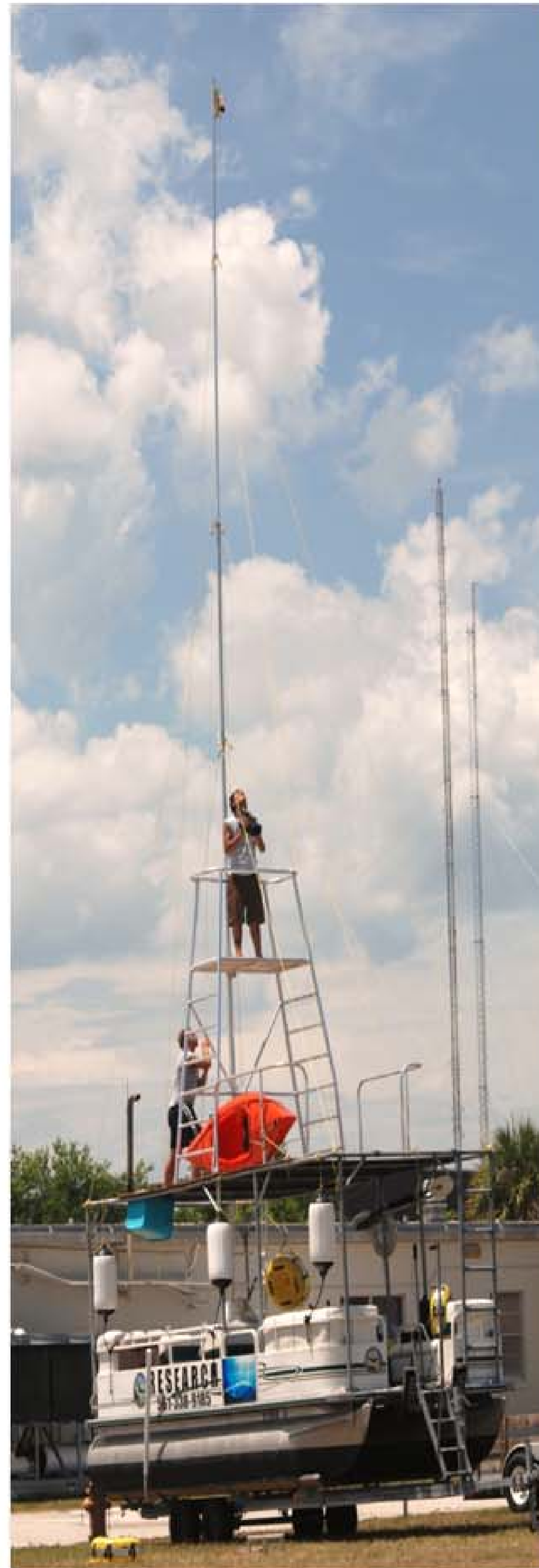
Figure 5. Pontoon boat with three observation decks and a 46ft video camera pole
