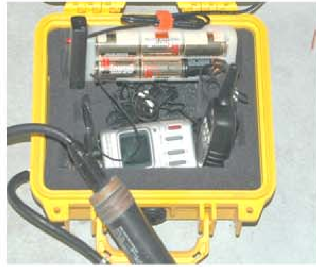
Figure 2a. DARP components: two channel digital flash card recorder, power sled, walkie talkie and hydrophone.
