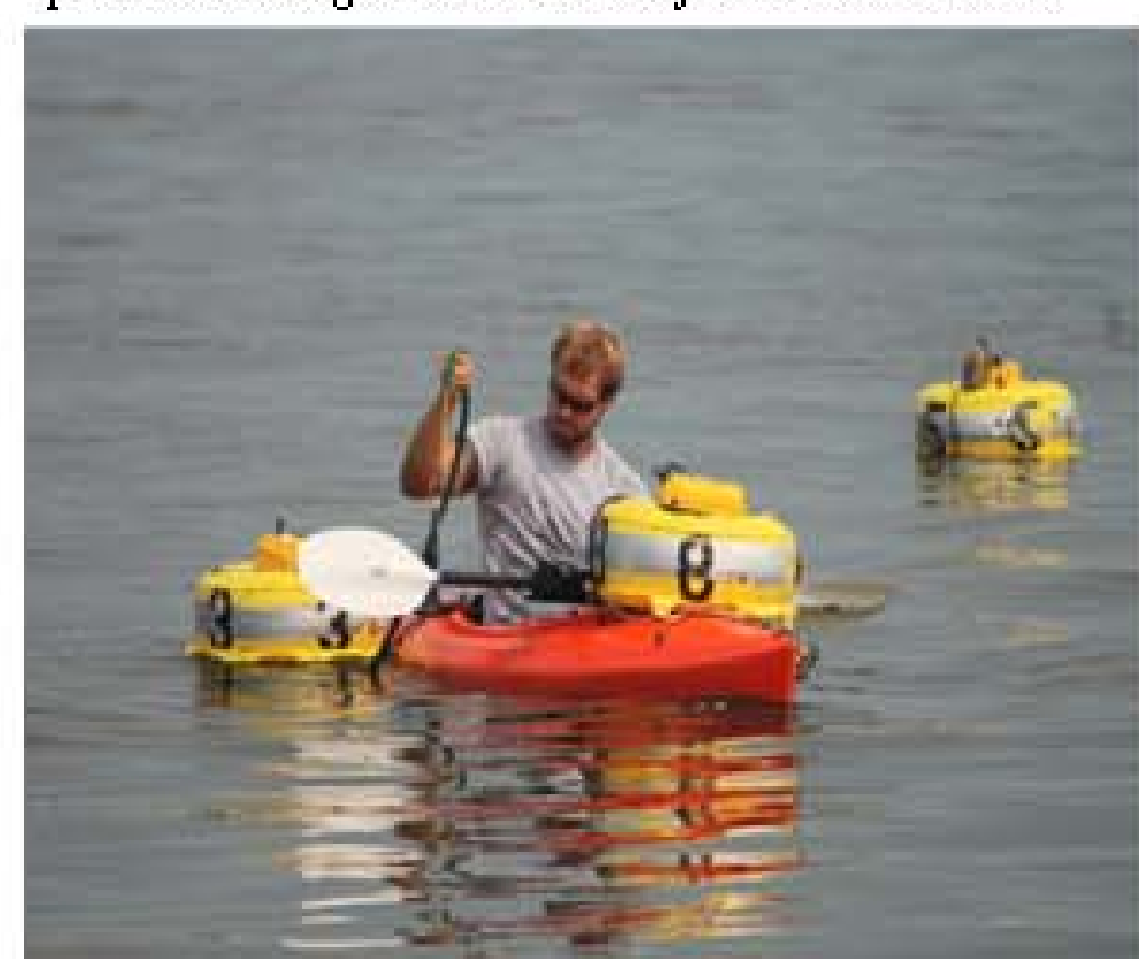
Figure 2c. Buoys were soft deployed using a kayak to minimize any possible disturbance to manatees in the area
