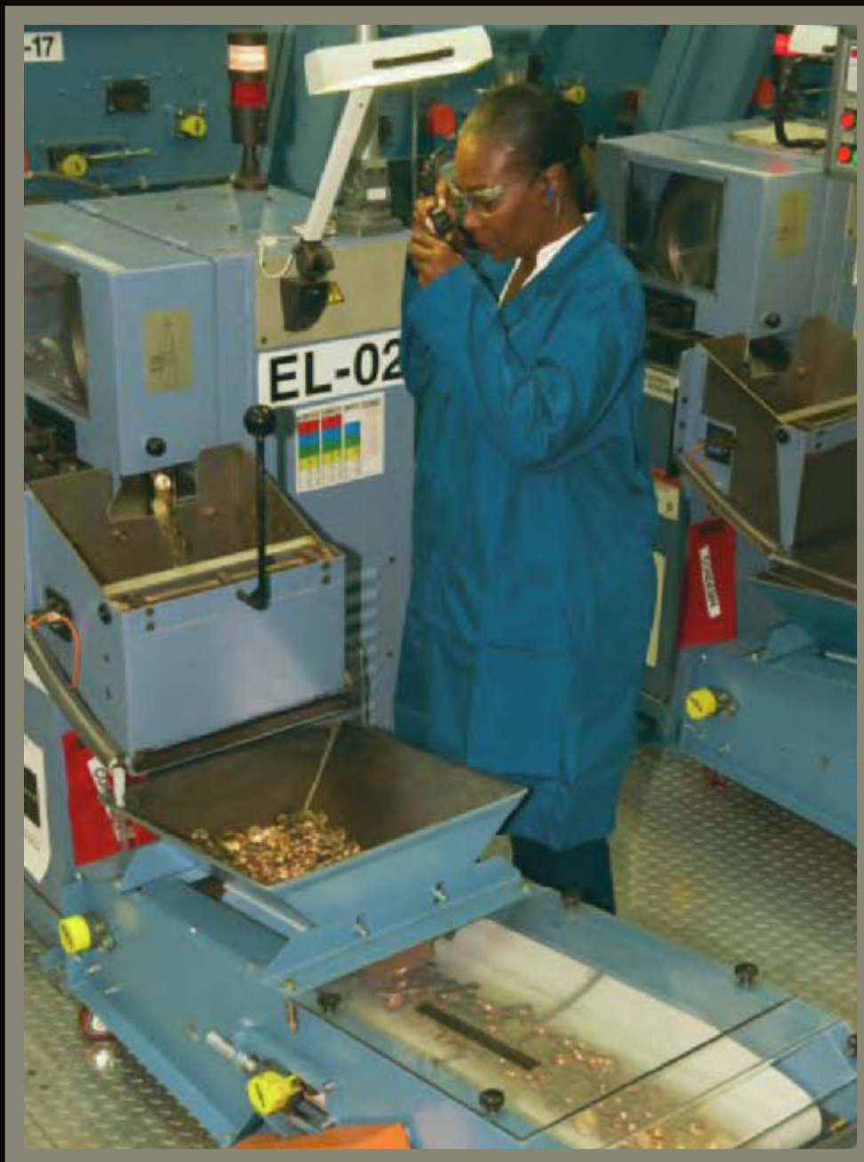
United States Mint at Denver employee Gail Frazier inspects the edge lettering on a Presidential $1 Dollar Coin. Edge lettering is applied after the coin is minted. Once the blanks are dried, they move to the upsetting mill. This machine raises rims around the edge on both sides of the blank and reduces it to a size that fits into the coining press collar.
