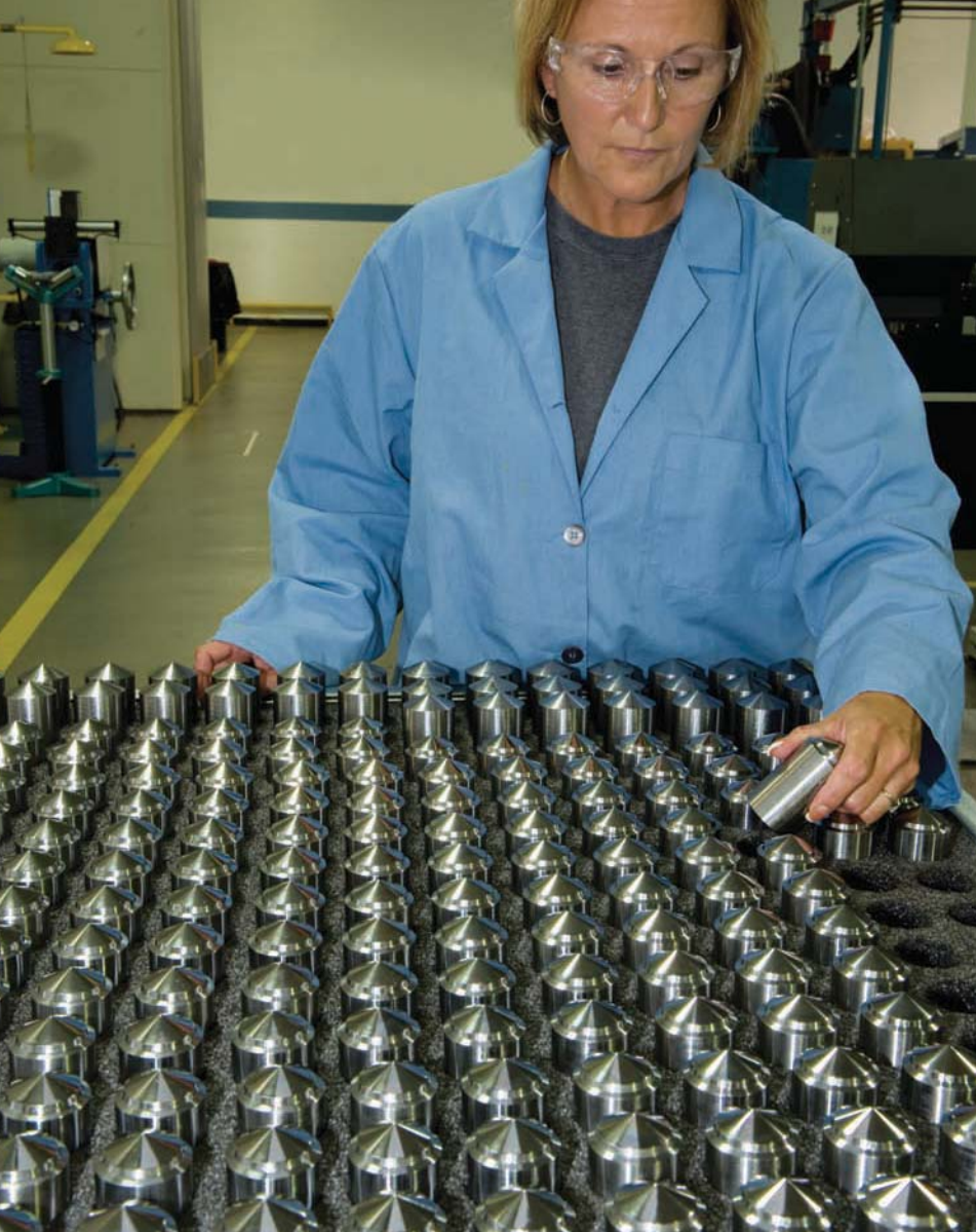
Cone-ended durable steel blank dies are inspected before the coin designs are hubbed (mechanically pressed) into the dies.
