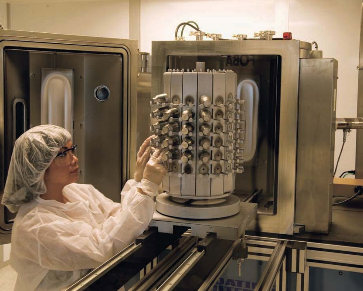
The physical vapor deposition coating system deposits a hard protective coating onto the surface of dies to extend die life and improve coin appearance.
