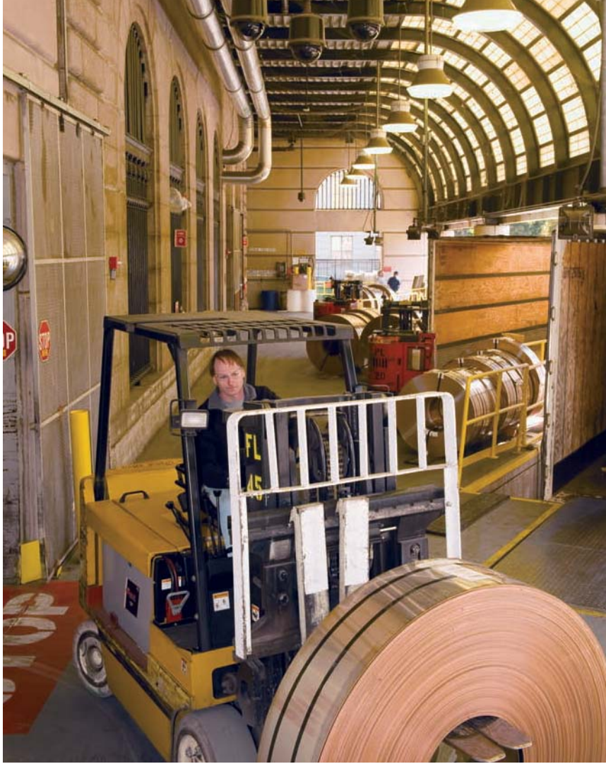
Most coin production starts with coil — rolled-up strips of flat metal. Operators transport and load coil onto a wheel that feeds into a blanking press. From the sheet, the blanking press punches out round, plain-surfaced disks called cut blanks.
