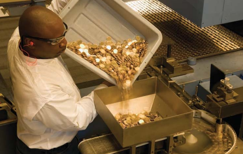
An operator at the United States Mint at Denver feeds $1 coin blanks into a weigh belt that feeds the annealing furnace, which softens blanks prior to stamping.
