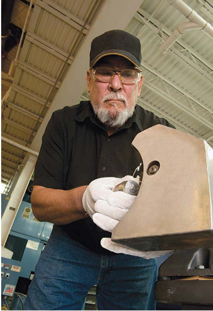
Dies for proof quality coins are hand polished at the United States Mint at Denver to improve coin appearance.
