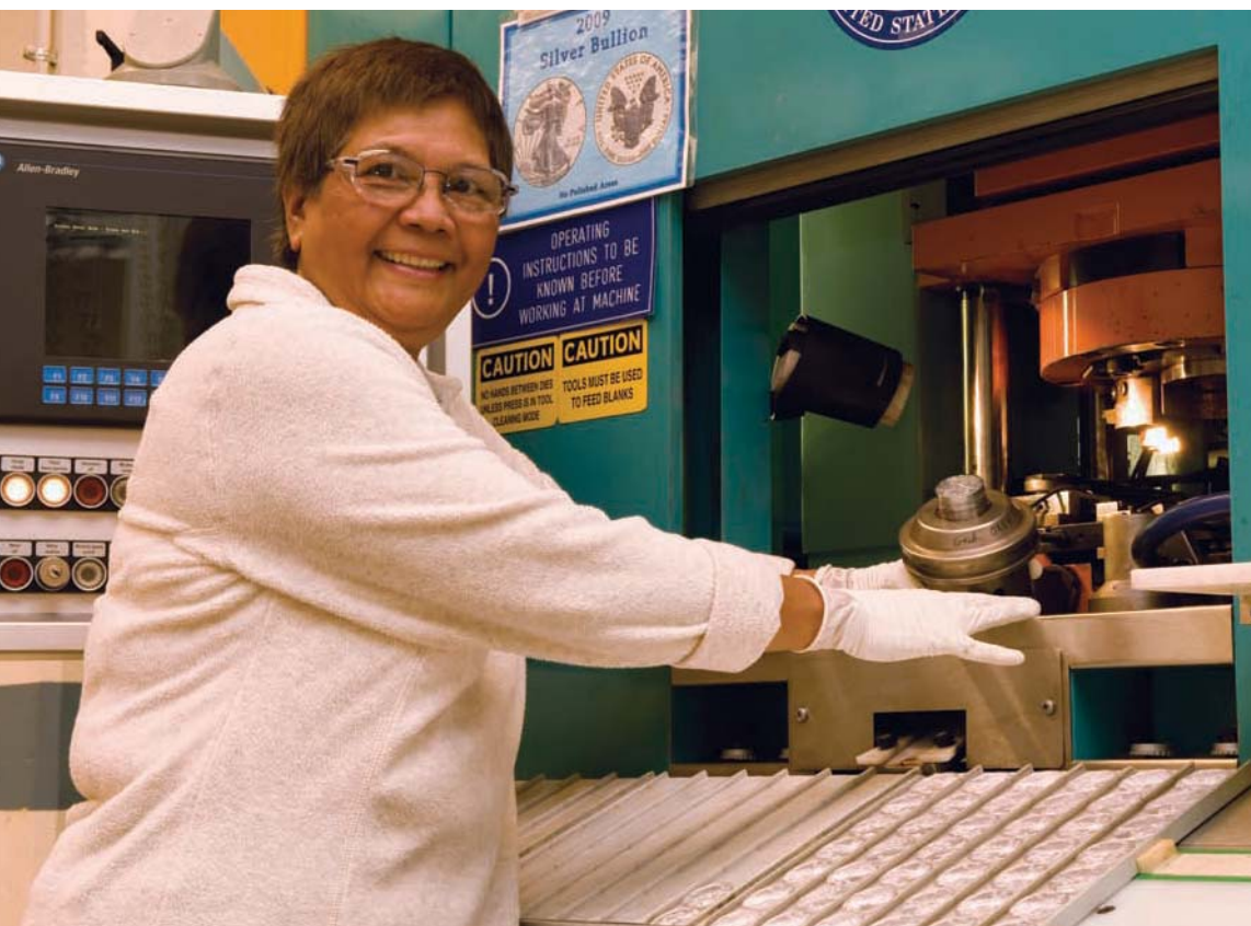
American Eagle Silver Bullion coins are minted at the United States Mint at West Point. The force of each stamping press is adjusted according to the blank’s size, hardness, design intricacy and relief.
