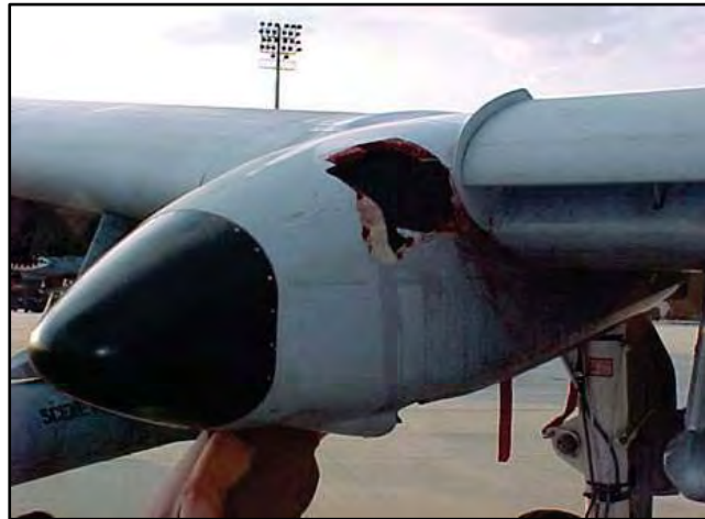
Photo of aircraft damage to an A-10 Warthog after colliding with an Osprey.
