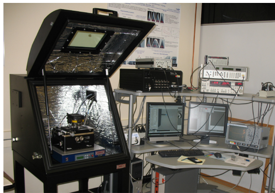
Contact-resonance force microscope system, used for highly localized measurements of elastic response in films and nanoparticles.
