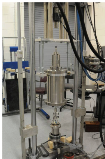
100kN fatigue test machine with 138 MPa hydrogen chamber.
