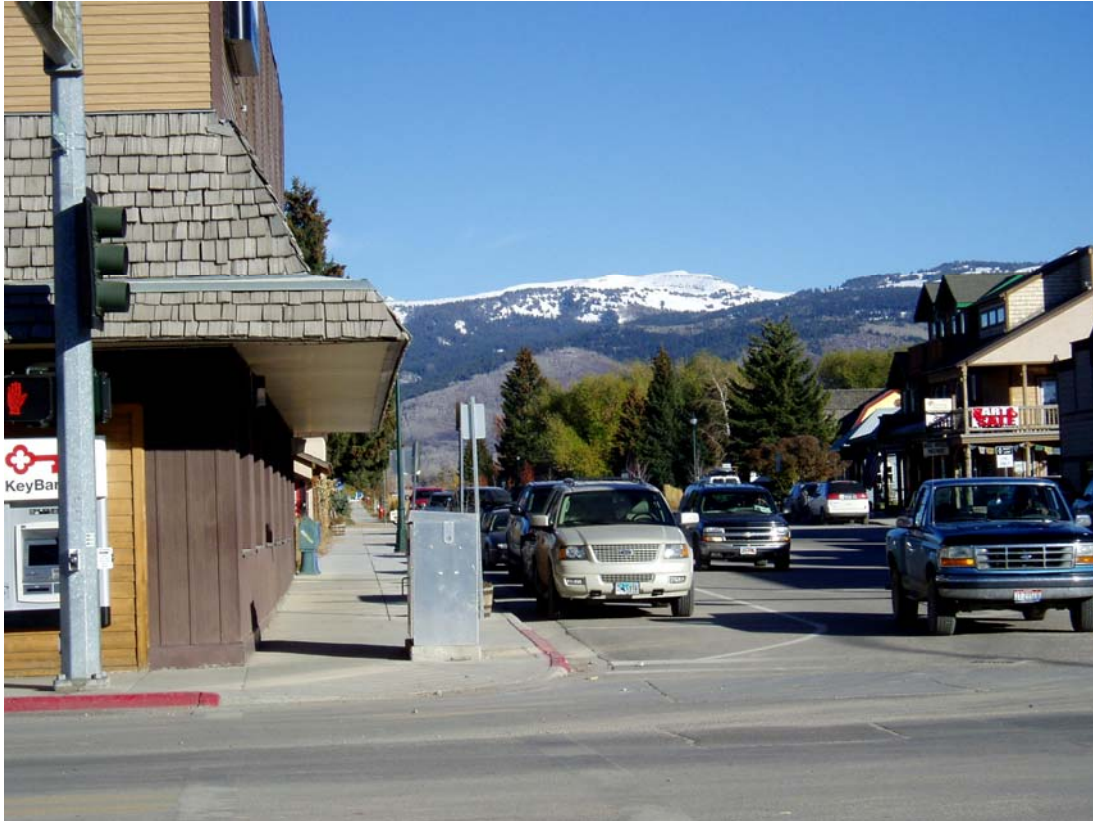
Figure 16: The corner of Main Street and Little Avenue in Driggs looking east showing the basic elements of the pedestrian realm – roadway corridor with parallel parking, room for a furnishing strip, sidewalk, and setback
