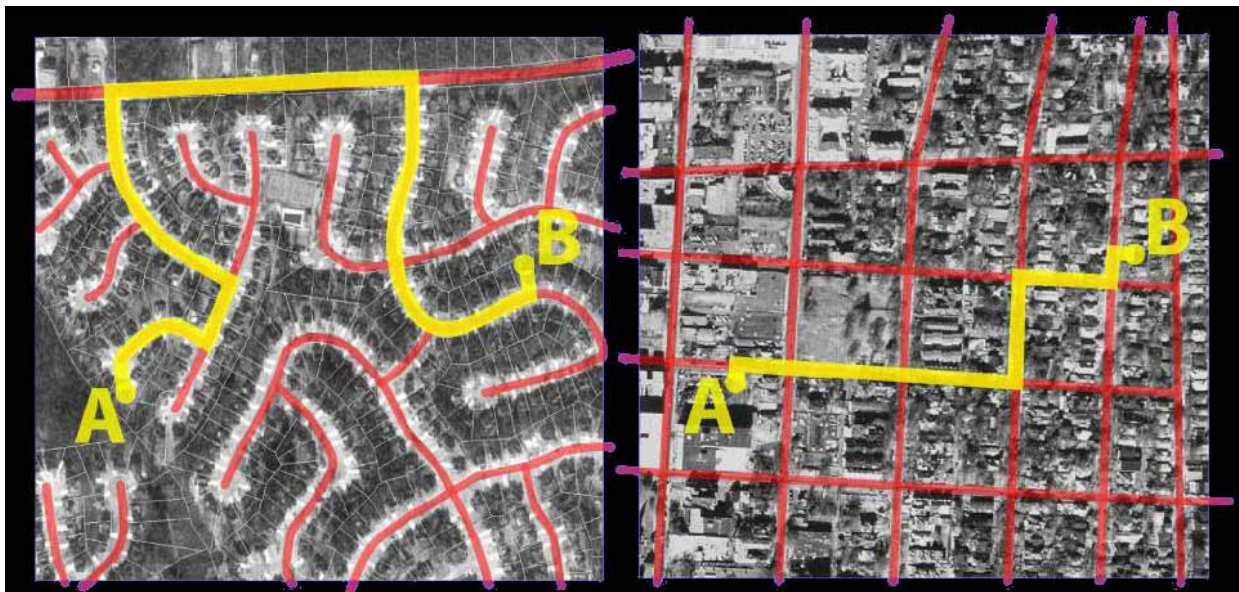
The image of the left depicts a poorly connected street network consisting of cul-de-sacs and pods of development. The image on the right shows a well-connected street network. Note the trip distance shown by the yellow lines. Longer trip distances discourage pedestrian activity and force people into cars for every errand.
