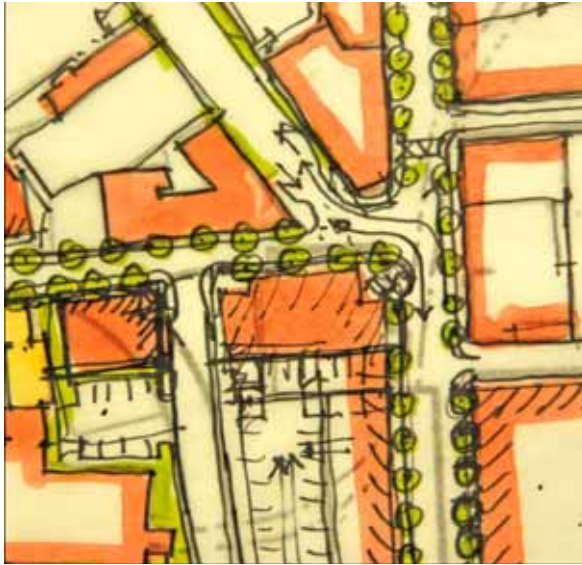
This rendering depicts a potential realignment of streets at the intersection of Beacon Street, West and Water Street. This approach reconnects Water Street with Main Street.
