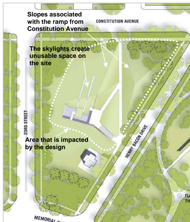
The diagram illustrates the area of the site that is impacted by the project's skylights, courtyard, walkways and associated slopes
