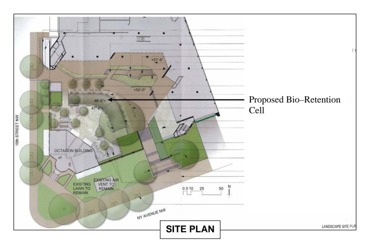
Addition sustainable design elements include a green roof on the lower roof, a bio-retention cell as indicated on the Site Plan, solar hot water collectors and a new "cool roof" membrane that has a high solar reflectivity. Rainwater will be collected from the main roof level and stored in a cistern on the parking level underground. This cistern will be used to reduce the building's use of potable water.
