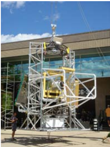
The Solar Bolometric Imager (SBI) shown here is an innovative, balloon-borne solar telescope that can take images in light integrated over nearly the entire solar spectrum.
