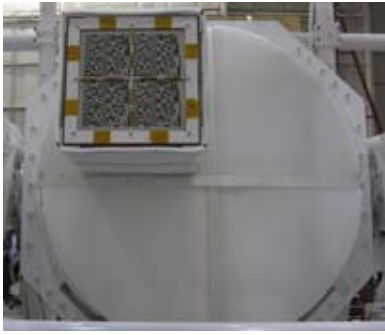
The front of ProtoEXIST1, showing the tungsten coded mask, which is essential for imaging at hard x-ray energies over a wide field of view.
