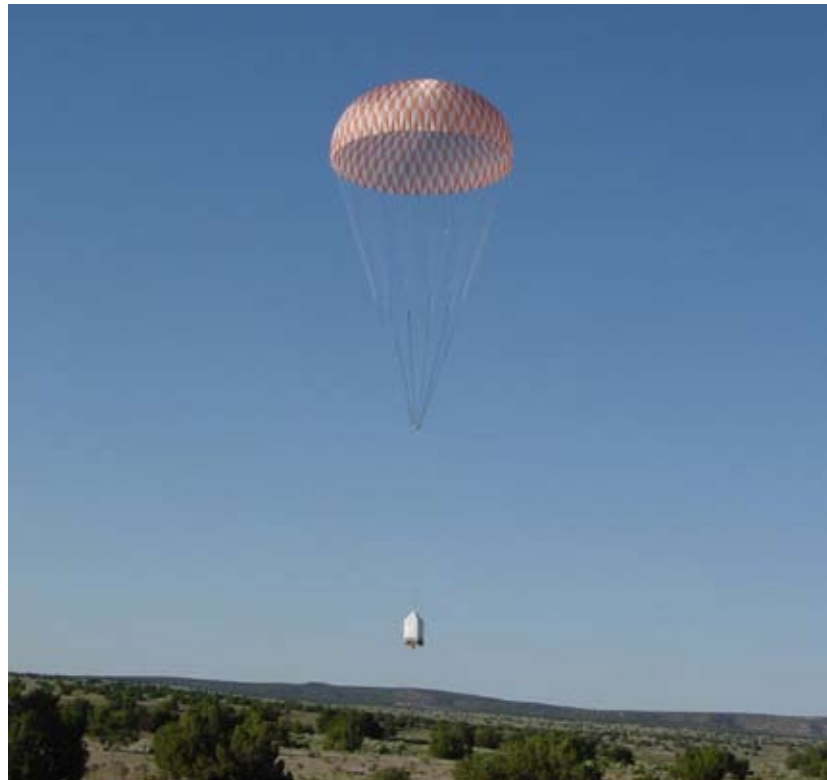
Touchdown for the Far Infrared Spectroscopy of the Troposphere (FIRST) experiment, in June 2005, after a successful flight. FIRST measures the radiation of the Earth in the 10–100 \mu regime.
