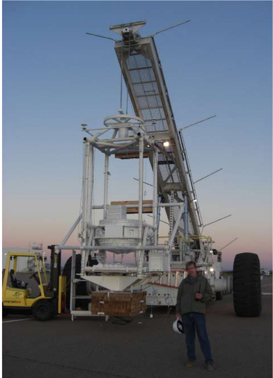
ProtoEXIST, a balloon borne instrument to develop technology for the Energetic X-ray Imaging Survey Telescope (EXIST) mission. EXIST is a candidate for the Black Hole Finder Probe and will conduct a census of black holes in the known universe.
