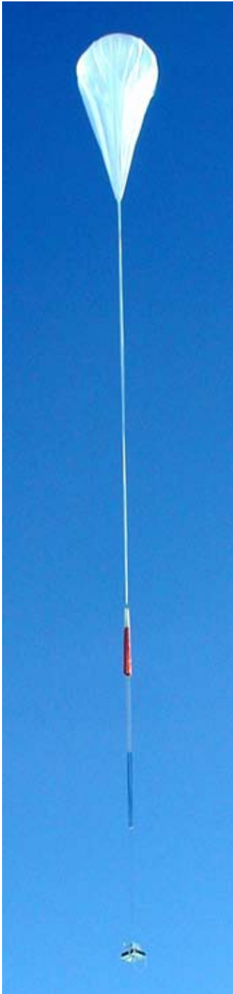
Shortly after launch helium fills only a small fraction of a balloon's volume. At float altitude the helium has expanded and the balloon is nearly spherical. (See image on page 28.)
