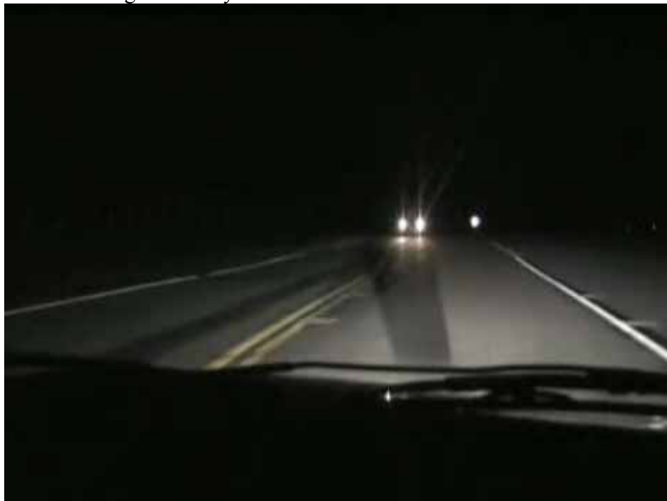
Figure II-13. View from the test vehicle toward an oncoming vehicle with the shielded prime beam installed.
