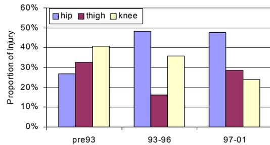
**Figure 13. Proportion of AIS 2+ knee, thigh, and hip (skeletal, joint, and ligament) injuries in different model years of air bag equipped vehicles.**
