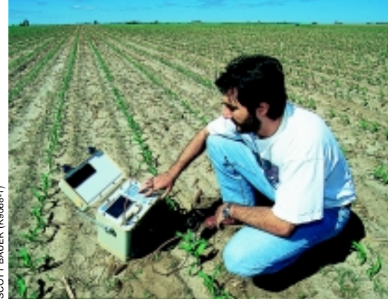
Cagatay Tanriverdi, CSU graduate student, monitors soil water content with a time-domain reflectometry probe.
