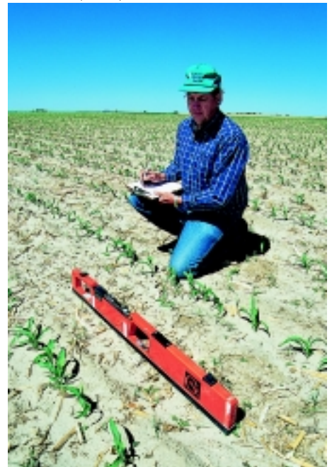
Agricultural engineer Gerald Buchleiter collects electromagnetic conductivity data to assess water and nitrogen levels in soil.
