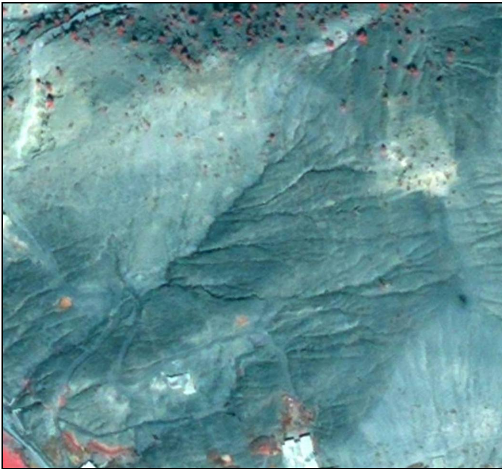
Figure 10-5 Active Gully Erosion (scale about 1:3000) (© DigitalGlobe)
