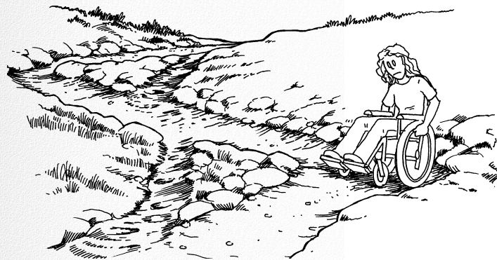
Figure 15-10. POTENTIAL PROBLEM: This switchback will result in difficult travel for wheelchair users because the slope is greater than 5 percent at the turning area.
