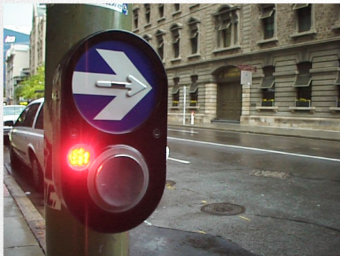
Figure 6-15. GOOD DESIGN: This pedestrian actuated signal device, used widely in Australia, provides information to pedestrians in audible, visual, vibrotactile, and tactile formats.
