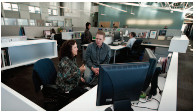
NREL’s Research Support Facility features open office spaces with low dividers to maximize the building’s use of available daylight.
