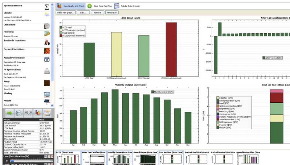
SAM's user-friendly interface is designed to help guide decision makers through the steps of analyzing the energy outputs and economics of a solar, wind, or geothermal project.
