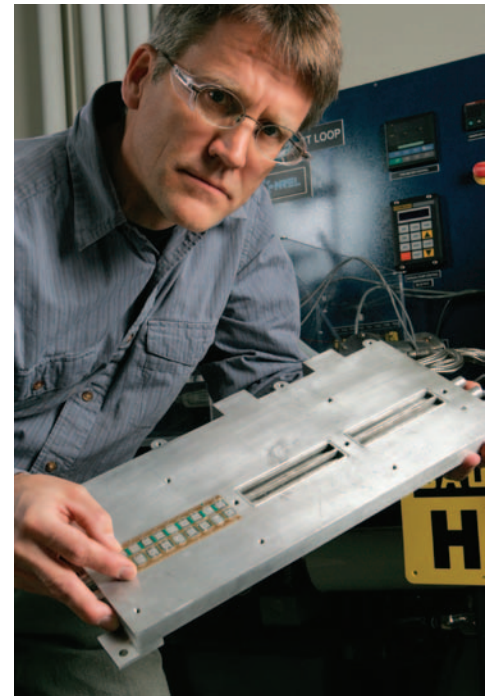
NREL researcher Ken Kelly holds a prototype cooling plate with built-in channels for liquid cooling of power electronics for the Semikron inverter. PIX 16916
