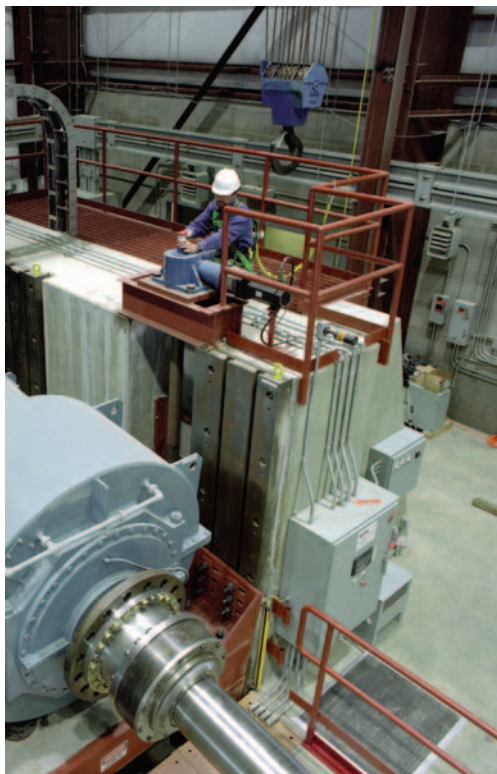
The 2.5-MW dynamometer test bed facility located at NREL's National Wind Technology Center PIX 08577
