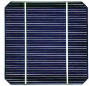
c-Si \sim 180 \text{ }\mu\text{m}
