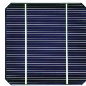
c-Si \sim 180 \text{ }\mu\text{m}
