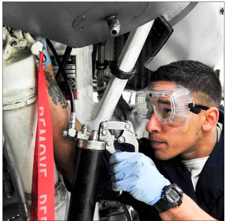
Senior Airman Christopher Blackstone, 51st Maintenance Squadron phase crew chief, applies lubrication to the nose landing gear struts of an A-10 here, March 7, 2012. Blackstone is applying the lubrication to ensure points are able to maneuver freely without corrosion. (U.S. Air Force Photos by Senior Airman Adam Grant)
