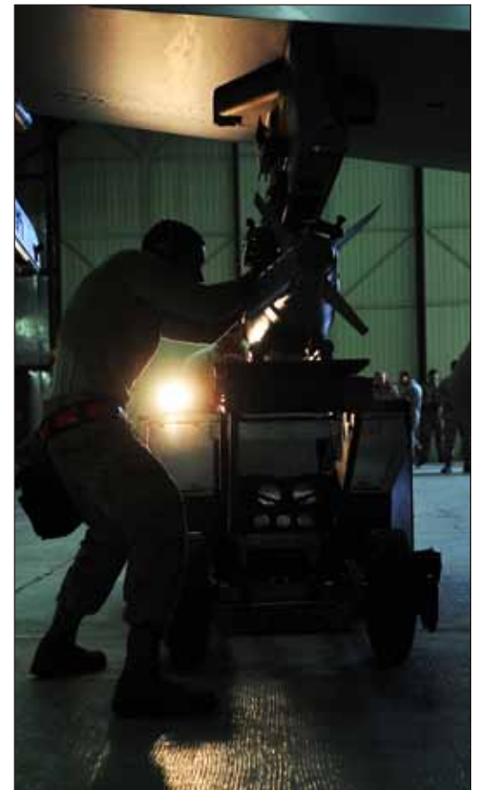
Above: Staff Sergeants Christopher DeGrizio (left) and Brian Crews, 25th Aircraft Maintenance Unit load crew members, work together to load a GBU-38 on an A-10 Thunderbolt II during the 4th quarter load crew competition here Jan. 20, 2012. The three-man team competed against the 36th AMU and won. They now compete against other load crews at U.S. Air Force bases in the Pacific. (U.S. Air Force photo by Staff Sgt. Craig Cisek)
