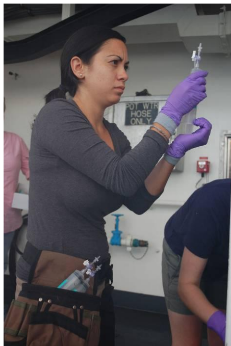
A researcher from the University of California at Santa Barbara checks a water sample for air bubbles on board the NOAA Ship Pisces during a September 2010 NRDA mission.
