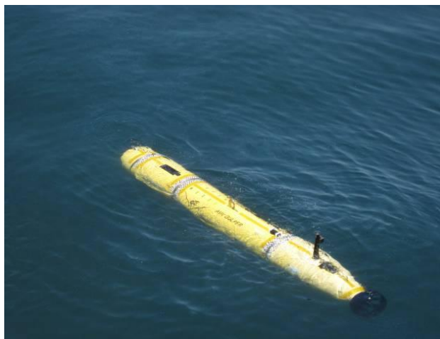
An Integrated Ocean Observing System glider is used to locate and track oil at various levels in the water column as well as on the water surface.
