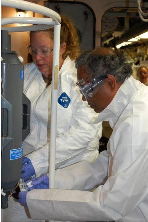
Researchers gather water samples from a rosette that measures CTD (conductivity, temperature, depth).
