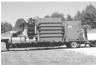
T-10 Donovan Blast Chamber safely detonates UXO in place.
