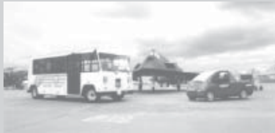
The F-117 stealth fighter sits between alternative fuel vehicles at McClellan Air Force Base, California. All 3 vehicles have something in common—they all use “composite” rather than traditional metal materials in their construction, making them lighter and more energy efficient.
