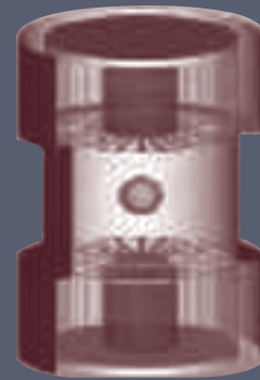
Schematic of a double-ended hohlraum with the deuterium-filled capsule at the center.
