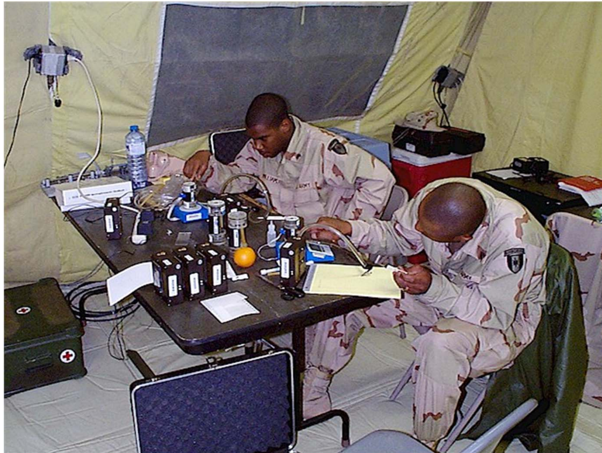
Area Medical Lab calibrating Personal Air Sampling Devices used in assessing Occupational and Environmental Health Exposures
