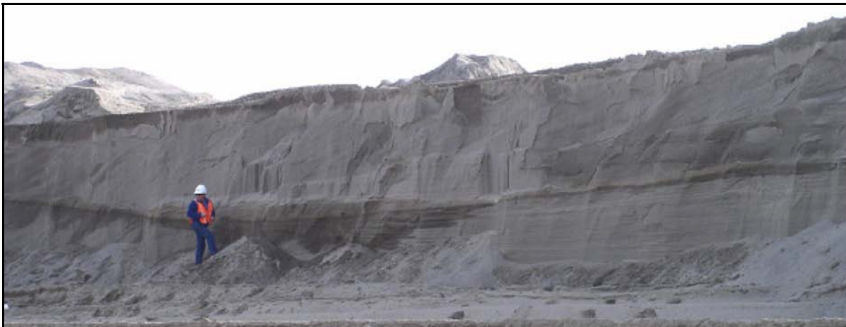
Figure A.10. Sand-Dominated Sediments of the Hanford Formation. This photograph is of a freshly cut sediment exposure at the Integrated Disposal Facility sited along the southern edge of the 200 East Area. (Source: DOE-RL 2008b)
