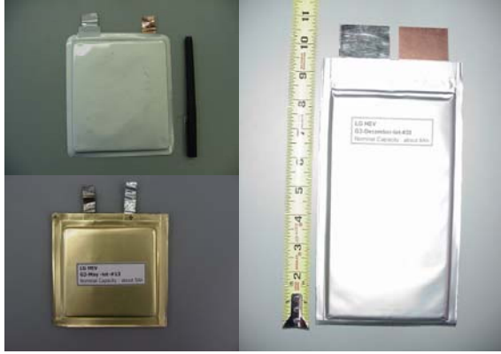
Figure 1: (Counterclockwise from upper left) CPI Gen I cell, Gen II cell, and Gen III cell.
