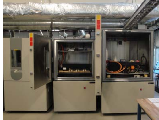
TTF laboratory environmental chambers (3/5) with JCS & A123 PHEV battery packs under test
