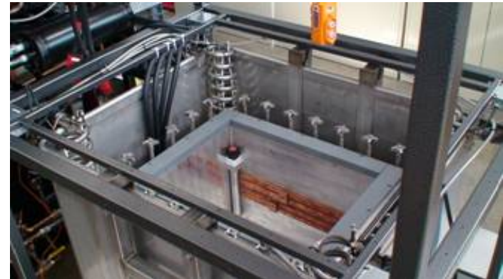
Calorimeter test chamber in isothermal fluid tank
