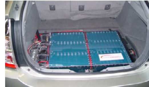
Bipolar pack in a Plug-In Prius
