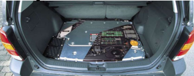
6.5 Ah HEV cells in Ford Escape HEV
