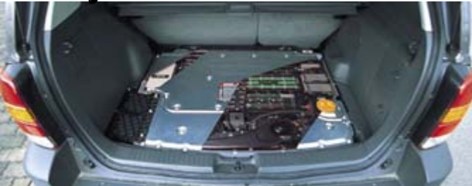
6.5 Ah HEV cells in Ford Escape HEV
