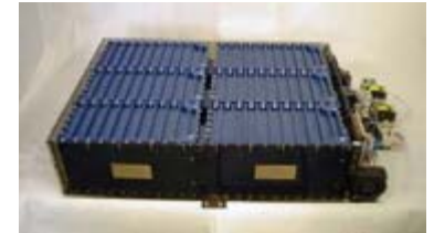
Pack with bipolar Cells/Modules
