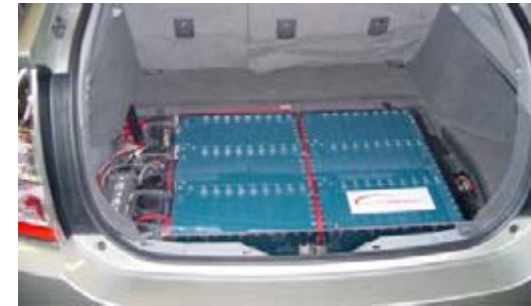
Bipolar pack in a Plug-In Prius
