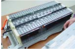
6.5 Ah Battery for Toyota
