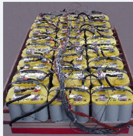
Optima battery pack used to test cycle life
