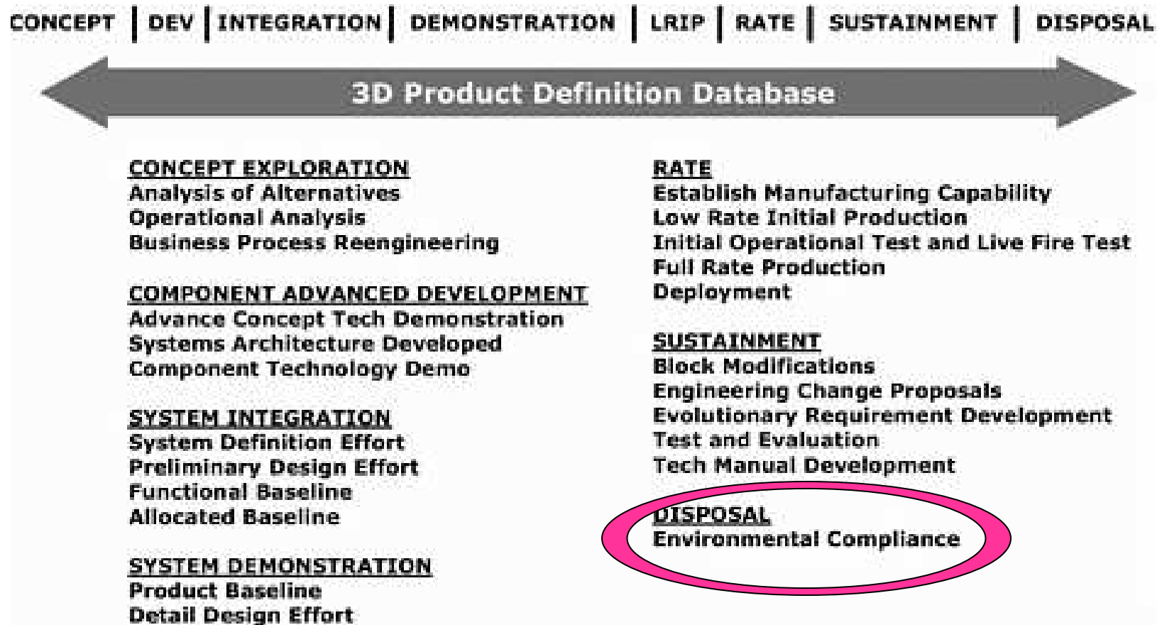
Figure 3-4 Life-cycle phases expanded into the eight indicated at the top of the figure.
