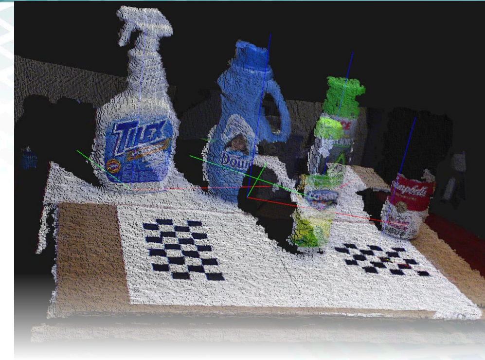
This “robot’s eye view” shows how some common household objects appear through the vision system being used in the Perception Challenge. The objects are fuzzy because the cameras have limited resolution. However, the images do provide information on depth (distance of every point on an object). The checkered patterns help to define and verify objects in space. (Credit: Courtesy Willow Garage)
