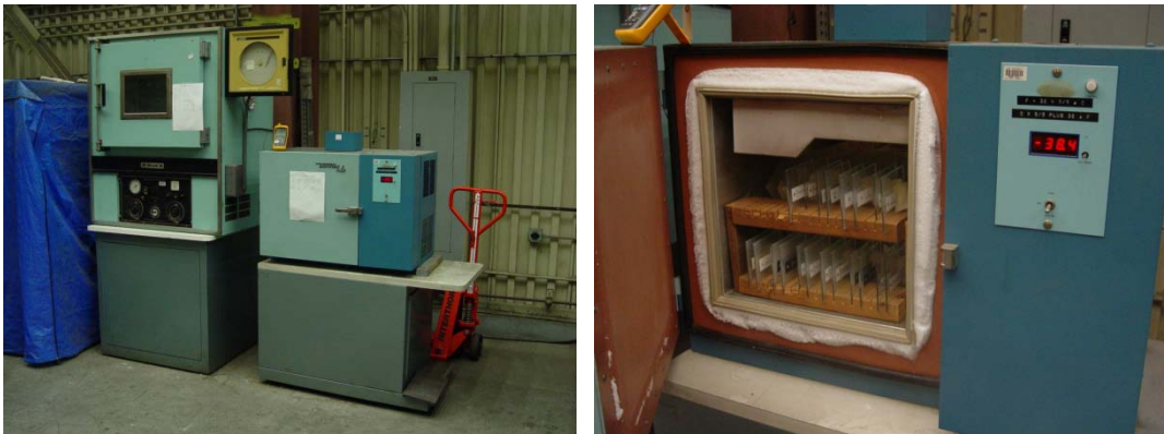
Figure 8. Environmental test chambers (left) and labels after a cold increment (right).
