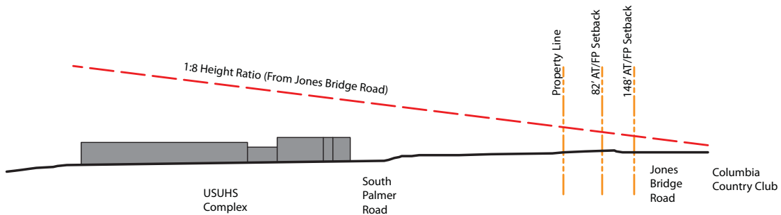
FIGURE 6-6 SECTION D- RECOMMENDED BUILDING ENVELOPE FOR SOUTHEAST CAMPUS AREA- VIEW TOWARD EAST
