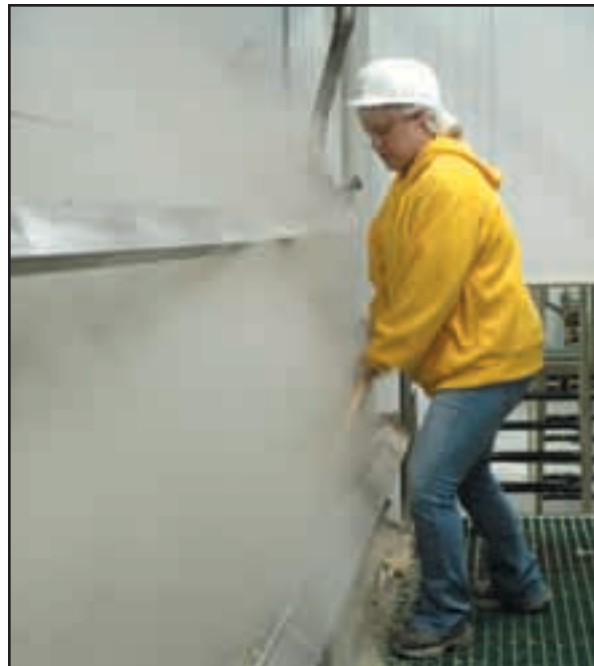
Potatoes are steamed during the dehydration process at the new Keystone Potato plant near Hegins, Pa., which uses power from methane gas piped in from a nearby landfill. USDA photo by Dan Campbell; Facing page: photo courtesy U.S. Potato Board
