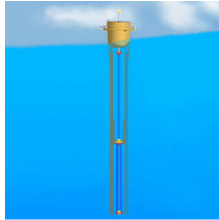
FIGURE 5 AquaBuOY Point Absorber Wave Energy Converter (Source: AquaEnergy Group, Ltd. 2005)
