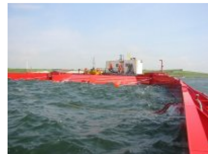
FIGURE 6 Wave Dragon Overtopping Device (Source: Wave Dragon 2005)
