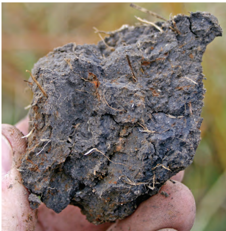
Figure 23. Redox features can be small and difficult to see within a dark soil layer.
