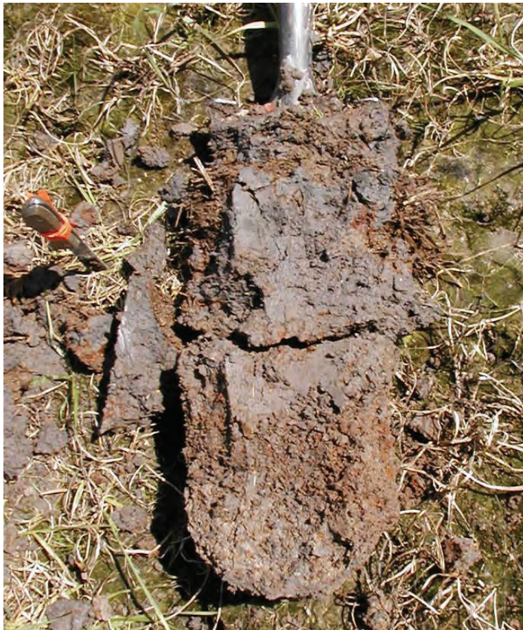
Figure 50. Redox concentrations in the tilled surface layer of a recently cultivated soil.
